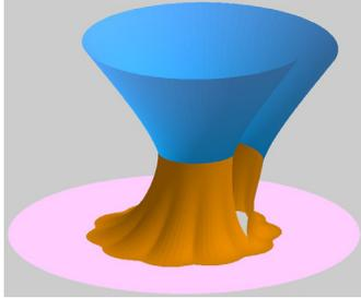
Figure 5: Blending between an open surface and a plane at a specified pedal-like curve.
