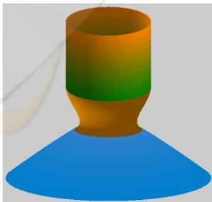
Figure 6: Blending between a circular cylinder and an elliptic hyperboloid of two sheets.
