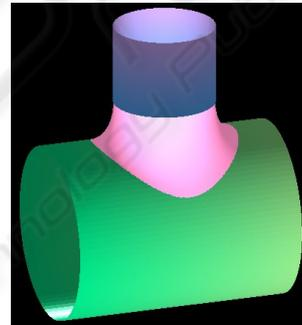
Figure 7: Blending between two intersecting cylinders.
