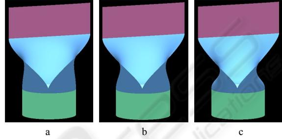
Figure 1: Different shapes of the blending surface created by different vector-valued shape control parameters.
