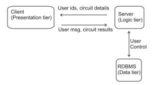
Figure 2: System architecture.
