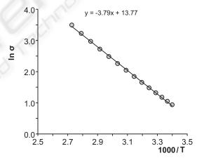
Figure 4: Plot of  $\ln \sigma$ :1000/T for the calculation of the energy gap of Ge crystals.
