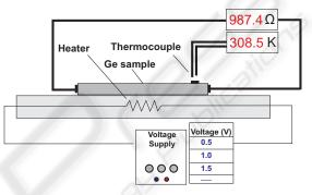
Figure 3: Typical circuit with a Ge crystal.
