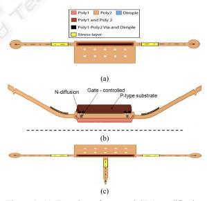
Figure 4: (a) Top view of proposed SDA modification from (Donald et al., 2006) in order to perform both left and right turn. (b) Frontal view of proposed SDA modification from (Donald et al., 2006) in order to control pull-in/snap-down voltage of the stylus steering arms. (c) Top view of proposed SDA modification from (Donald et al., 2006) in order to include micro-scalpel.
