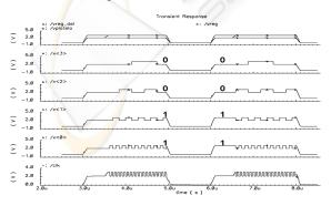
Figure 8: Simulation result of 4-bit counter.
