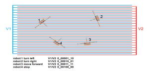
Figure 10: V1 / V2 are used as channels to apply binary encoded controls to each micro-robot.
