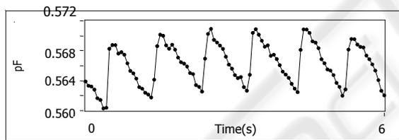
Figure 3: Capacitance measurement for electrodes mounted on the finger.
