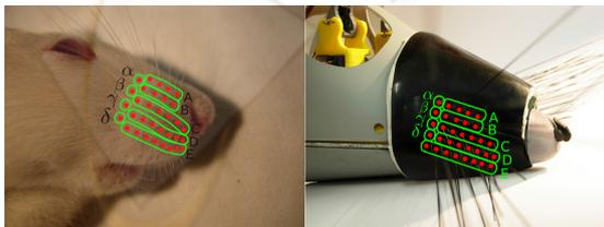
Figure 1: Comparison of whisker pads in a real rat and in our robot.
