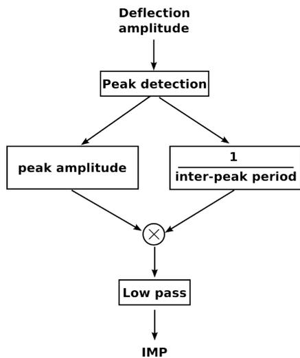
Figure 2: Feature extraction algorithm. "Peaks" are detected through the monitoring of the signal's derivative and frequencies are estimated through the inverses of the time intervals between successive peaks. Then, the peak amplitude is multiplied by the peak frequency, averaged within a time window.
