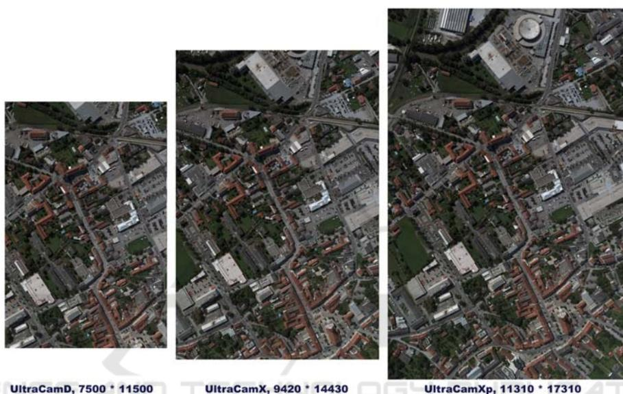
Figure 1: Image formats of the UltraCam-versions D, X und XP. Obviously, a larger format will increase the efficiency of image collection resulting in fewer aircraft flight miles and fewer individual images and data files.
