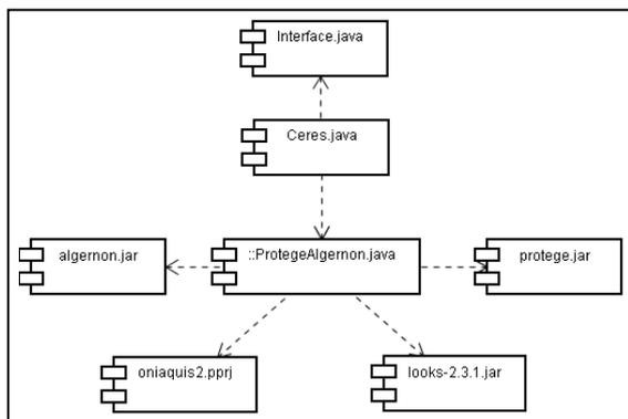
Figure 2: Component's Structure.
