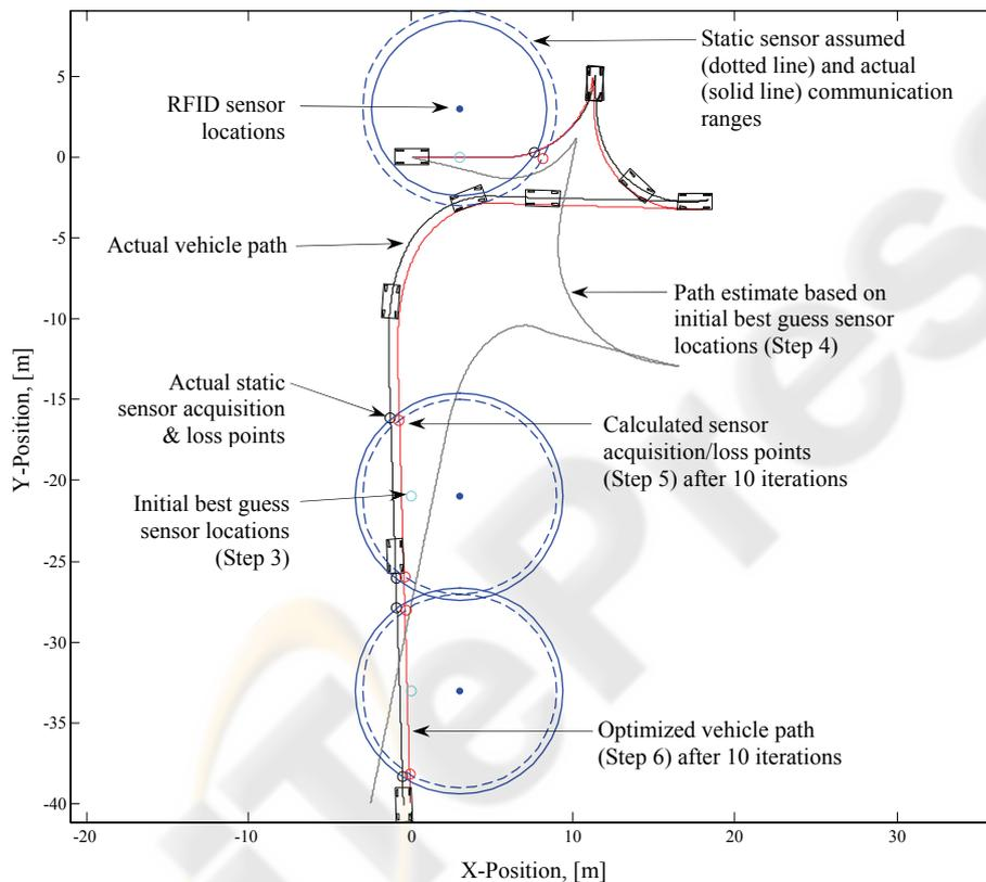
**Fig. 3.** Forklift path reconstruction showing actual forklift position evenly spaced in time, RFID antenna locations and ranges, initial path estimate, and final path estimate after ten iterations.
