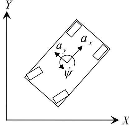
**Fig. 2.** IMU signals and axes.
