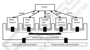
Figure 4: Hosting environment architecture.
