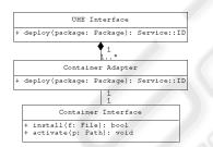
Figure 3: Design pattern notation of container abstraction.
