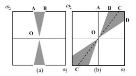
Figure 1: Ideal wedge filters specified in the frequency plane: (a) along the axis  $\omega_2$ ; (b) oriented at an angle  $\varphi$ .
