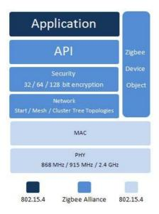
Figure 2: ZigBee stack architecture.
