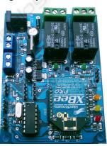
Figure 6: Sensor and actuator board.
