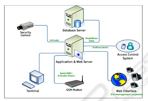
Fig. 1. An overall layout of the elderly monitoring system.
