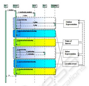
Figure 1: Sequence diagram with tangled behaviour due to crosscutting concerns.
