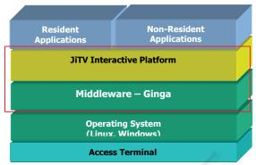
Figure 1: Architecture of the JiTV Platform.
