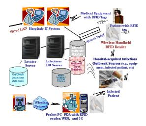
Figure 1: Main components of RFID-enabled HIODMS Architecture.
