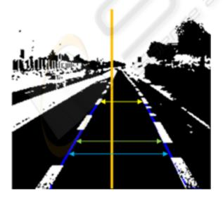
Figure 4: Horizontal distances between left and right points.
