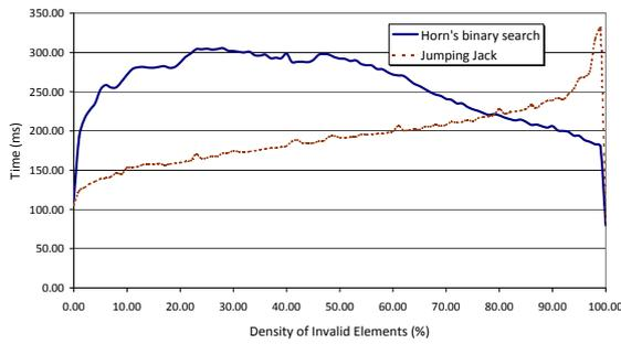
Figure 11: Overall time spent for compaction of a 4M stream by the two tested algorithms, versus the invalid elements density. A block size of 256 was used.
