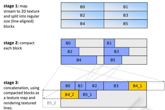
Figure 8: *Block Based Compaction* implementation.
