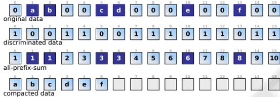
Figure 5: Compaction of a stream based on the all-prefix-sum.
