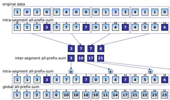
Figure 4: Segmented Parallel Prefix Sum for a stream with  $s = 16$  elements and segments (blocks) with  $b = 4$  elements.
