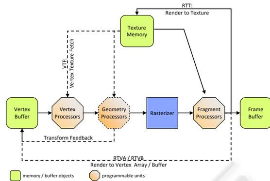
Figure 1: Simplified GPU programmable pipeline (as exposed by OpenGL). Dotted units and paths have limited / non standard support.
