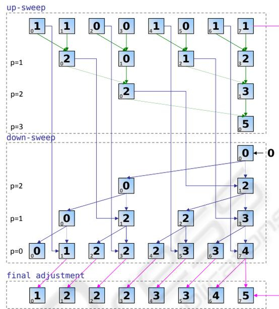
Figure 3: Parallel Prefix Sum using a balanced binary tree algorithm (after (Blelloch, 1990)) for a stream with  $s = 8$  elements.
