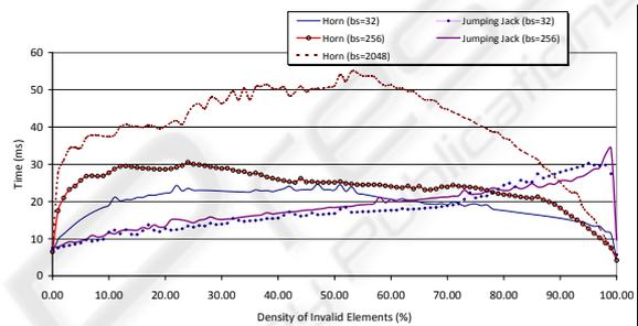
Figure 13: Timings taken on a nVidia GeForce 9500M GPU for intra-block compaction of a 4M stream versus the invalid elements density (*bs* denotes the block size)
