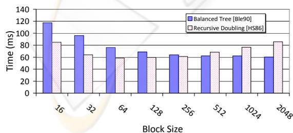
Figure 9: Timings achieved for intra-block block prefix-sums for a stream with 4M elements.
