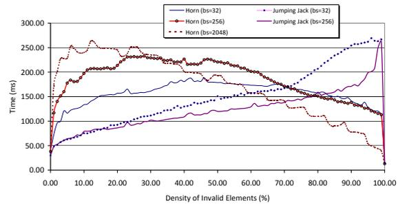
Figure 12: Timings taken on a nVidia GeForce Go 7300 GPU for intra-block compaction of a 4M stream versus the invalid elements density (*bs* denotes the block size).
