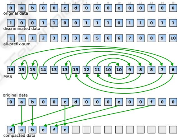
Figure 7: Graphical trace of the Jumping Jack algorithm.
