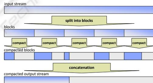
Figure 6: The *block based compaction* approach (after (Roger et al., 2007)).
