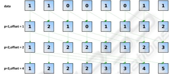
Figure 2: Parallel Prefix Sum using a recursive doubling algorithm for a stream with  $s = 8$  elements.
