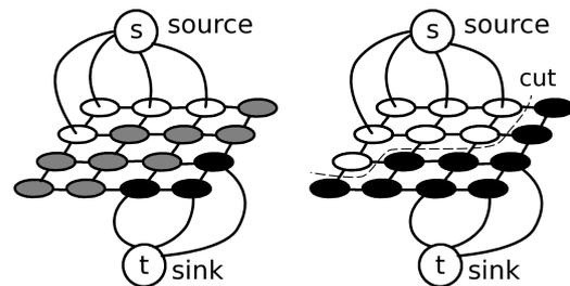
Figure 2: Principle of graph cut segmentation. Left: Initial state of the graph. Right: A cut on the graph.
