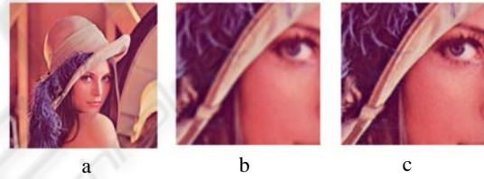
Figure 5: subsampled image of 512x512 pixels is shown in (a), a 4x magnification, using bilinear algorithm (b) and our method which produces more defined images (c).
