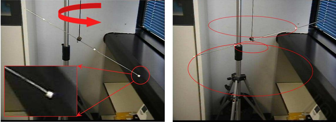
Figure 3: Simple 1D calibration tool. Notice that in principle any object with unknown geometry could be used, since the technique relies only on feature tracks. On the right are shown the three ellipses fitted from the tracked features.
