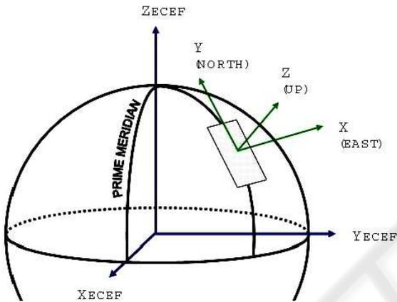
Figure 1: A plane tangent to the hypothetical spheroid surface contains the local East North directions, which set those axis for the East-North-Up reference frame.
