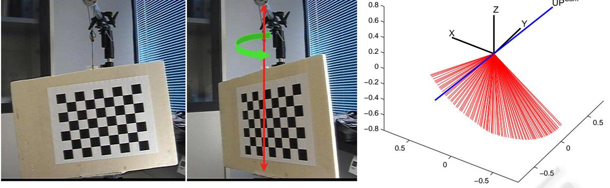
Figure 2: The two frames on the left show the rotation of the calibration planar object about the vertical direction, used as basic calibration step. The plot on the right shows an example of vertical direction estimation in camera reference frame, using the horizontal plane spanned by the vector  $\mathbf{Z}^{Cam}$ , normal to the calibration object, during one single-axis motion. In blue is drawn the vector  $\mathbf{UP}^{Cam}$  estimated by linear regression.
