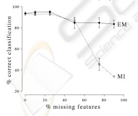
Figure 2: Example 1 of ML research on varying missing values. Classification of the iris data from (Ghahramani and Jordan, 1994).
