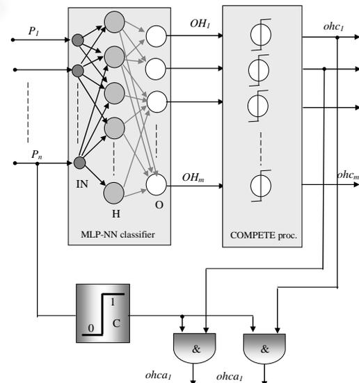
Figure 1: Obesity-Hypertension Neural Network Processing Scheme (ohcm – obesity-hypertension classes, ohca1, ohca2- obesity-hypertension additional classes).
