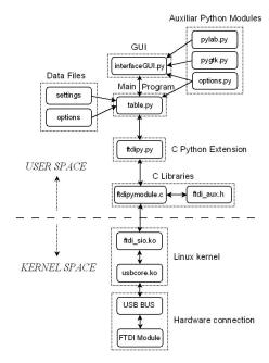
Figure 2: Software structure.
