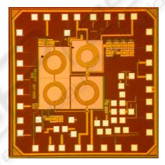
Figure 4: A die photograph of the RF transceiver.
