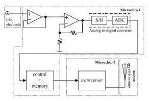
Figure 2: Wireless EEG module. Note that the neutral electrode, which is connected to the grounds of the module it is not shown.
