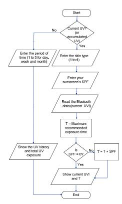
Figure 3: Software operation (it receives the new UV index each 15 seconds and stores to average for each hour).
