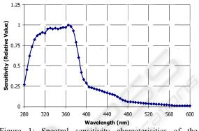
Figure 1: Spectral sensitivity characterisitics of the ML8511.
