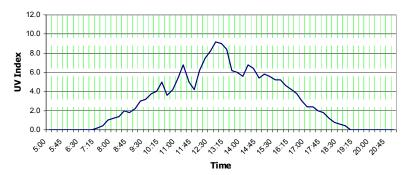
Figure 4: Example of personal UV monitor software (UV index was updated each 15 seconds throughout a partially cloudy day).
