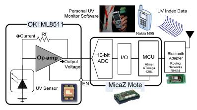
Figure 2: Schematic diagram of the personalized UV monitoring system.
