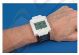
Figure 1: Wrist fall detection system.
