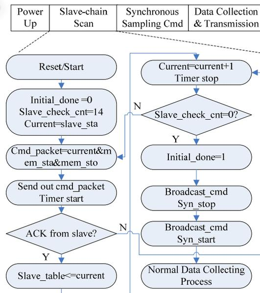
Figure 2: Slave-chain scan process.
