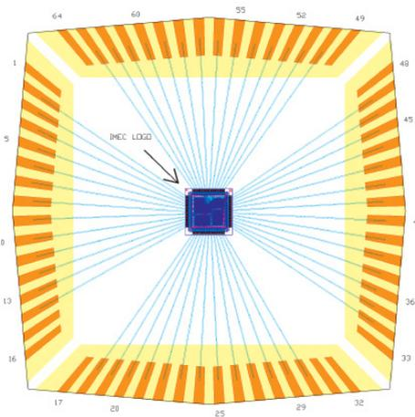
Figure 4: Package bonding diagram.
