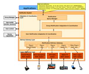
Figure 3: Architecture of the adaptive notification enabler.
