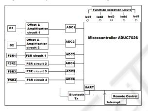
Figure 1: System block diagram.
