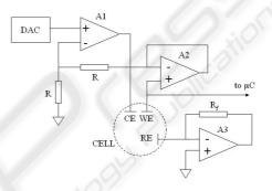
Figure 2: Potentiostat circuit.
