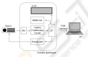
Figure 1: Block diagram of the instrument.
