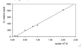
Figure 6: Linear calibration of lactate biosensor.
