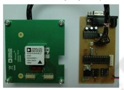
Figure 1: A photograph of the data logger system (right) and a miniature gyroscopes and accelerometers (left).
