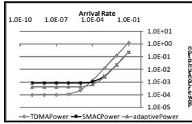
Figure 2: Power Consumption for the S-MAC, Ad\_Li, and the TDMA schemes, as a function of packet arrival rate for a random 1000 node topology.
