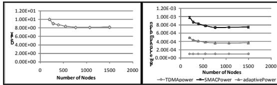
Figure 3: Delay (a) and power consumption (b) for the S-MAC, Ad\_Li and TDMA schemes, for topologies with increasing nodes, and no traffic.
