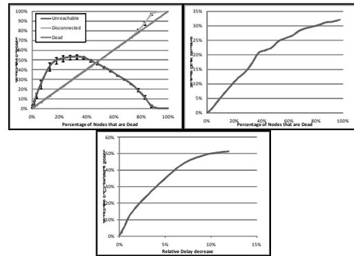
Figure 5: (a) The percentage of disconnected and unreachable nodes in the networks for varying numbers of dead nodes (1000 node topologies, 98% confidence interval). (b) The relative decrease of the end-to-end sensor to gateway delay (of the active nodes) in the networks for varying numbers of dead nodes (1000 node topologies). (c) The percentage of unreachable nodes in the network versus the relative decrease of the end-to-end delay (1000 node topologies).
