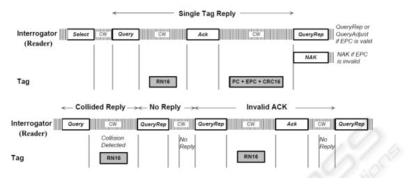
Figure 3: The proposed tag identification mechanism using CRC-16 and having different time duration for success, idle, and collision.
