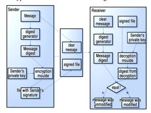
Figure 2: Principles for the realization of data integrity and non-repudiation.
