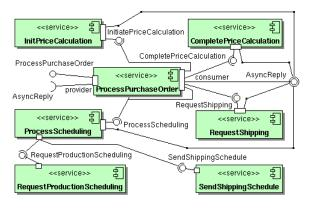
Figure 2: An overview of identified services, their interfaces and connections.
