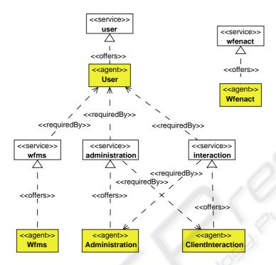
Fig. 2. Dependencies of the distributed workflow management system in development.
