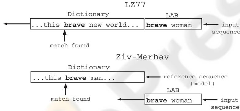
**Fig. 1.** The original LZ77 algorithm uses a sliding window over the input sequence to get the dictionary updated, whereas in the Ziv-Merhav cross parsing procedure the dictionary is static and only the *lookahead buffer* (LAB) slides over the input sequence.
