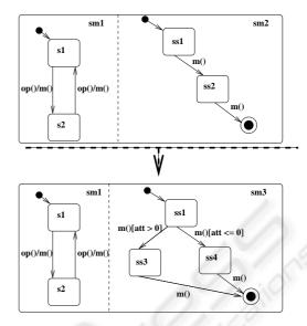
Figure 2: Refining a supplier state machine.
