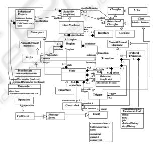
Figure 1: UML behaviour metamodel.
