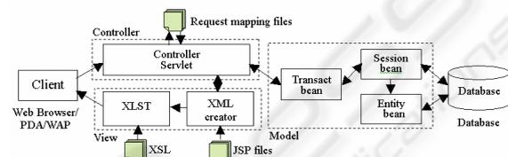
Figure 2: Extended MVC-based web application framework.
