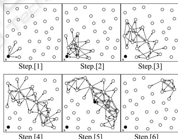
Step[1] : A source node transfer the data to every node in a range.
