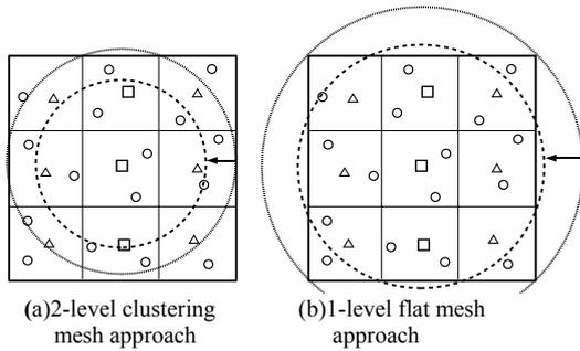
Figure 10: Restricted range in (a) 2-level clustering mesh and (b) 1-level flat mesh approaches.
