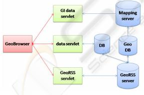
Figure 1: The system architecture.
