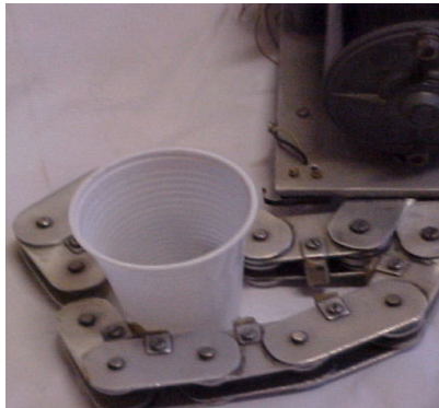
Figure 3: The hyper-redundant gripper of the arm.
