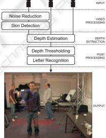
Figure 2: Scheme of the depth based drawing game.
