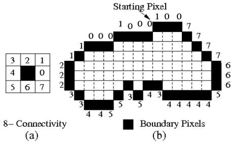
Figure 1: Example: Assignment of Boundary Chain(BC) codes.
