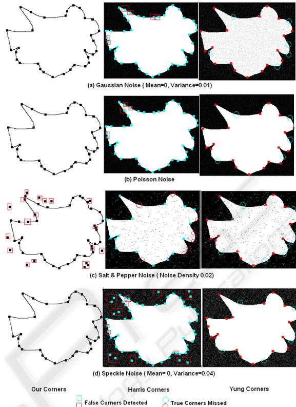
Figure 6: Corners extracted on noisy images (a) Gaussian Noise, (b) Poisson Noise, Salt-n-Pepper Noise, (d) Speckle Noise.
