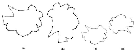
Figure 7: Transformation invariance of corner extractor(a) Original (b) Rotated by  $90^\circ$ , (c) Scaled 50% and Rotated  $180^\circ$  (d) Scaled 50%.
