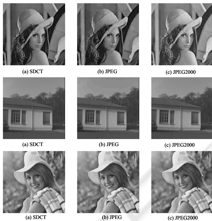
Figure 7: Coding quality performance of (a) SDCT (b) JPEG and (c) JPEG2000 codecs for 'Lena', 'Elaine' and 'House' test images at compression ratio of 40.
