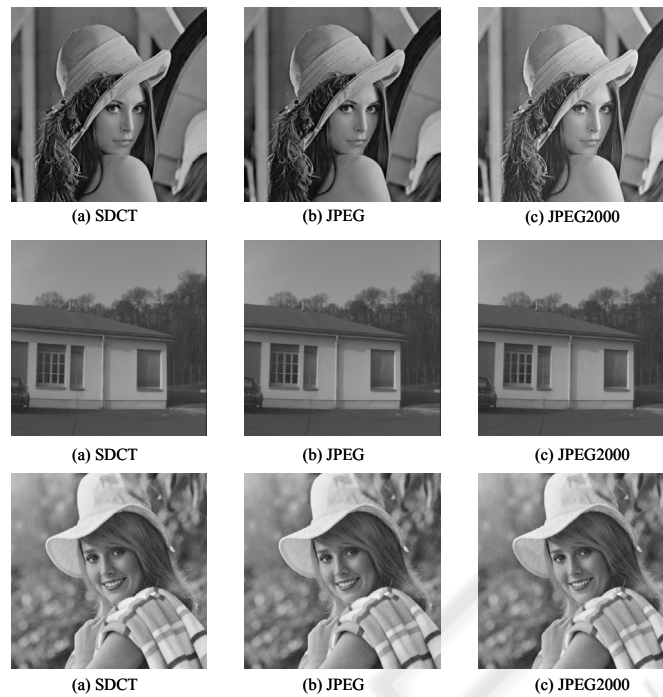
Figure 5: Coding quality performance of (a) SDCT (b) JPEG and (c) JPEG2000 codecs for 'Lena', 'Elaine' and 'House' test images at compression ratio of 5.
