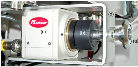
Figure 6: Low-cost camera system based on a door peephole lens (a) adapted to a CCTV camera (c). A mounting frame (d) is used to lock the peephole in a calibrated distance to the camera lens (b).
