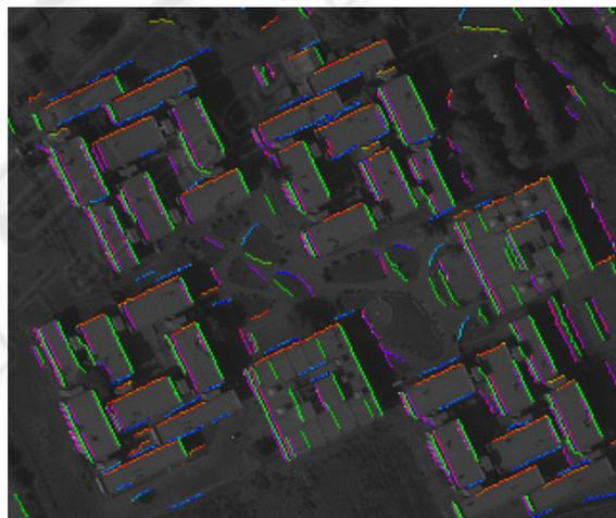
Figure 1: Segments highlighted in left image with colour based on orientation.
