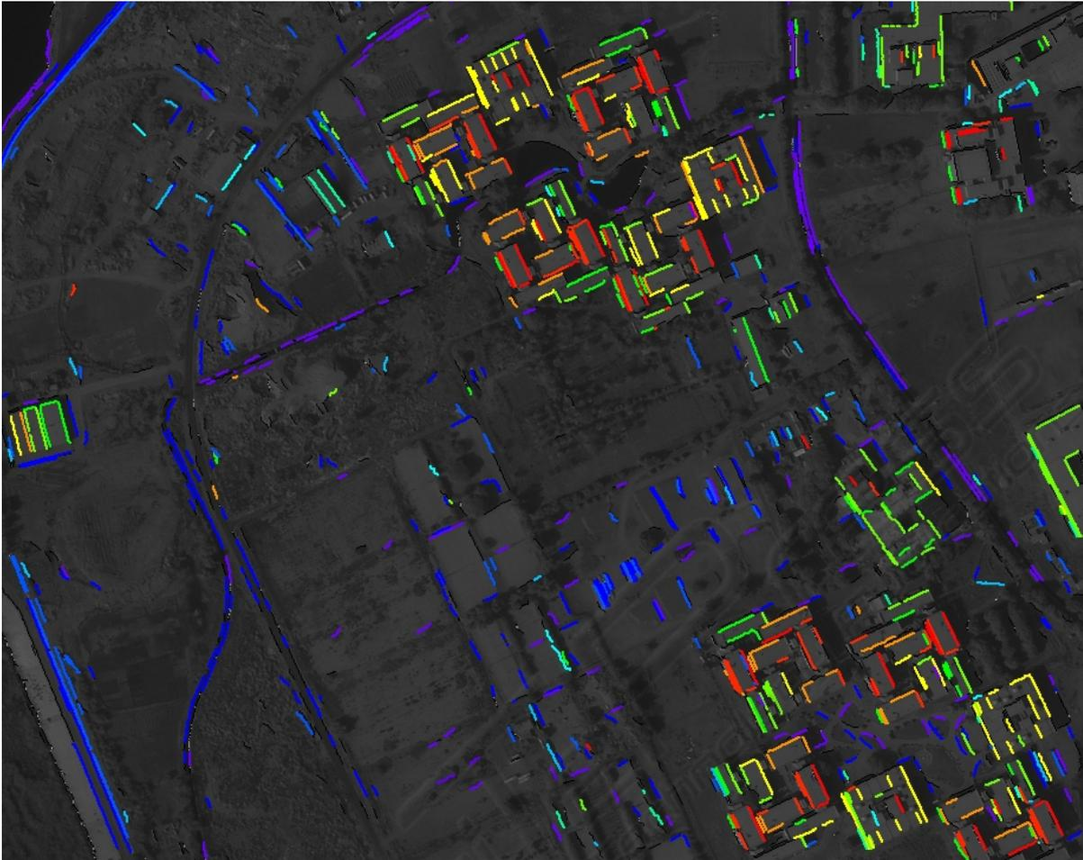
Figure 2: Display of matched segments with rainbow palette. Low segments are in violet and dark blue, medium in light blue and green and elevated segments are in yellow, orange or red.
