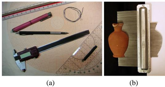
Figure 3: Tools for drawing a profile line: (a) pens, scale paper, lead-wire, ruler and sliding calliper, (b) *Profilkamm*.
