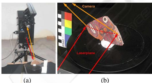
Figure 2: In-situ setup of the 3D-scanner (a) consisting of a Laser, a CCD camera and a rotational plate for acquisition of (b) e.g. a NASCA sherd found in the Valley of Palpa, Peru.
