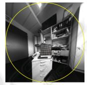
Figure 5: Correction of the radial distortion for a fish-eye lens. Left: The original fish-eye image in which the central area is denoted by the circle. Middle: The area inside the circle is transformed to the perspective model using the initial values for the internal camera parameters. The transformation is not correct since the scene lines are not straight in the image. Right: The area inside the circle is corrected using the estimated parameter values. The images of lines are straight.
