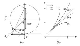
Figure 1: (a) A generic model for a central catadioptric camera (Ying and Hu, 2004). The Z-axis is the optical axis and the plane Z=1 is the virtual image plane. The object point  $\mathbf{X}$  is mapped to  $\mathbf{x}$  on the virtual image plane. (b) The projections (6)-(10) and their approximations with models (12) and (13).
