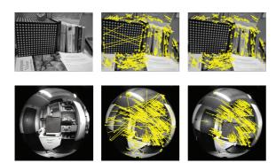
Figure 4: Self-calibration of a conventional (top) and a fish-eye camera (bottom) using the generalized catadioptric camera model. The tentative correspondences are illustrated in the second view (middle), where the flow vectors indicate several false matches. The last column shows only the inliers detected during the self-calibration.
