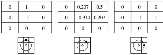
Figure 3: Filters  $F_1 \dots F_3$  of the total of 8 local derivative filters at (8,1) neighborhood. The remaining 5 filters are obtained by mirroring the filters shown here.
